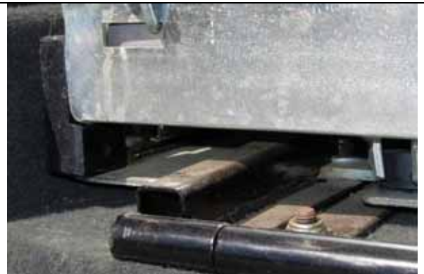
RHS welded on flat to reinforce & prevent flat bending instead of hinging. You could make the whole hinge frame out of RHS. I would next time.
