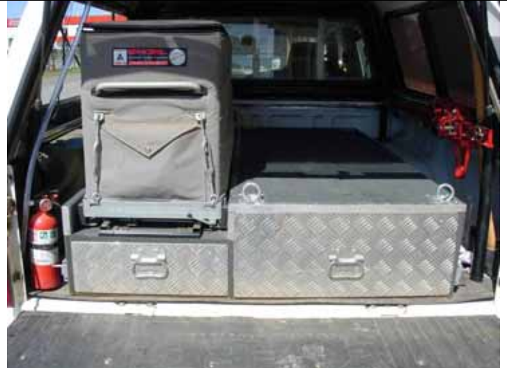
Closed – checker plate is wider than drawer front to cover slides
