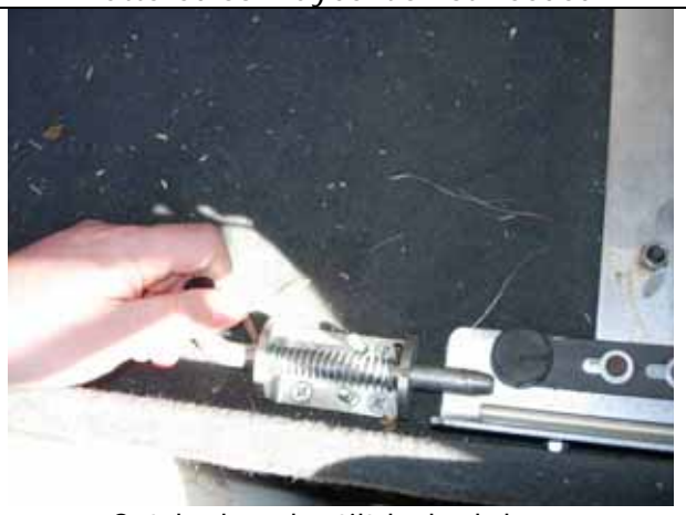
Catch closed – tilt locked down
