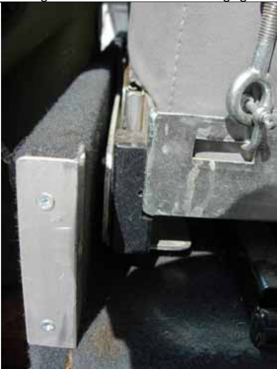
Clearance either side of fridge slide – not much. Sliders run inside gal angle so gal angle just has to clear box side to allow tilt action.
