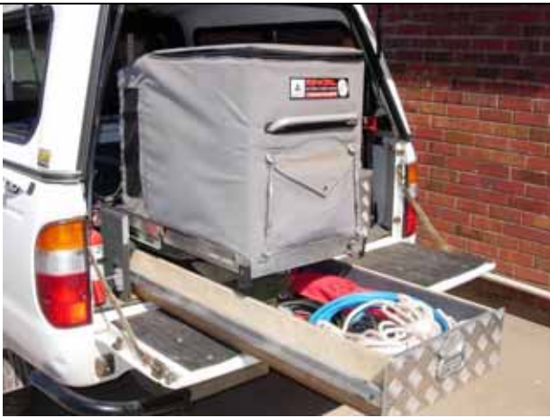
Fridge out with tilt lock still engaged
