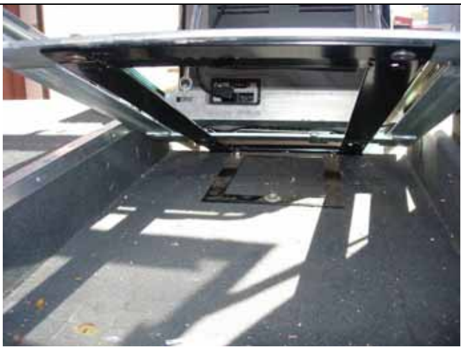
Hinge frame from underneath – note bolted up from inside drawer, using countersunk cap screws to stop drawer contents grabbing bolt heads.
