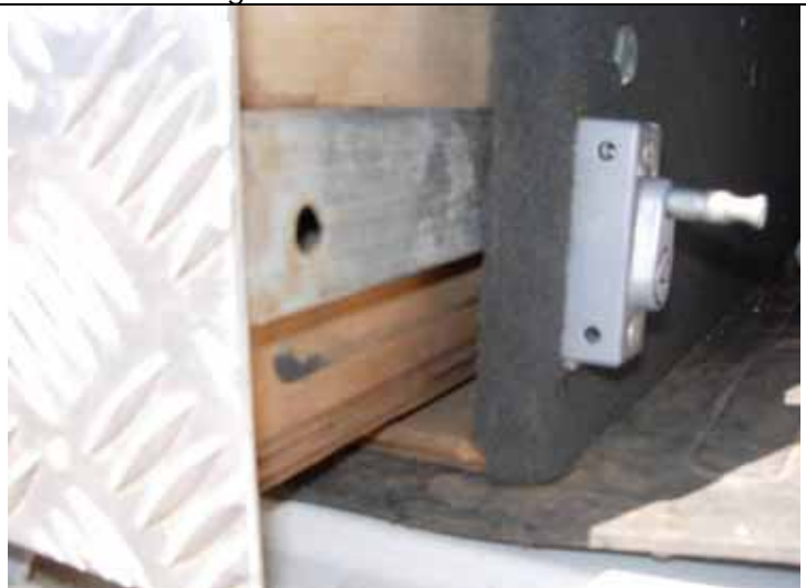
Window sash lock and hole in slide rail
