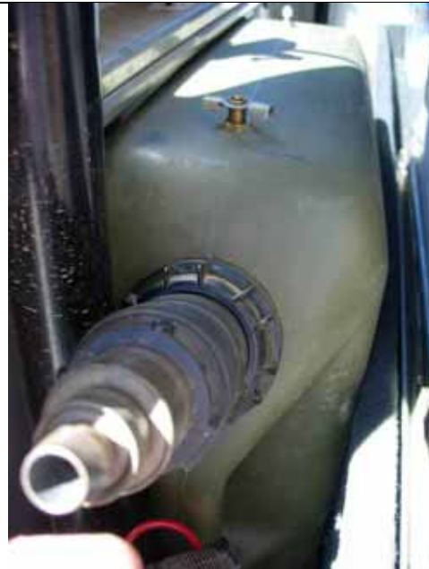
Bleed valve in top of tank.
