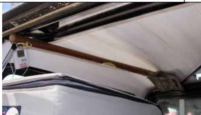
Shovel mounts up there too. Bracket for mouth of shovel welded on front bar. Locating pin and clevis clip hold handle
