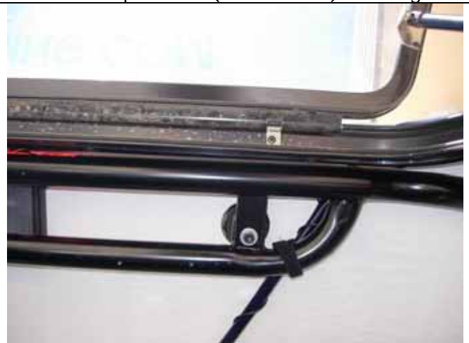
Bottom of a roof rack mount. Spare HF radio tapped whip too.
