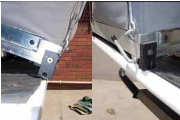
Nylon blocks act as bumpers on tailgate to clear slide lock mechanism in down position. Drilled & tapped fridge frame to bolt on.
