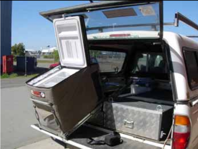
Full tilt with lid held open by clip to window rod
