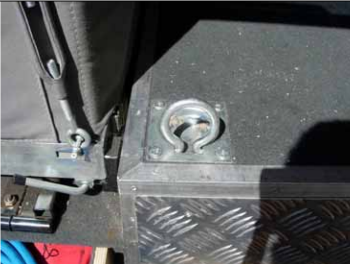
Tie down and alum corner stripping
