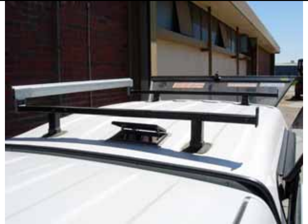
Roof bars – made them too. Gal bar is topped with sail track for awning, and another bit plugs in to front to extend it over cab. Awning goes all way to a removable pole on bull bar. Vent for pressure (reduce dust) and dog.
