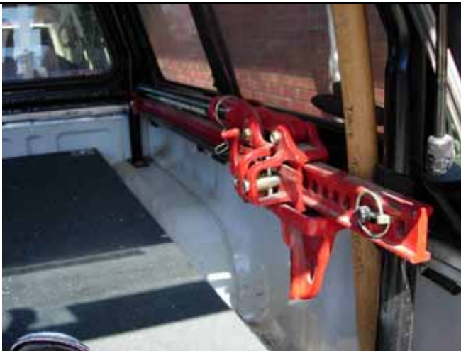
Jack mounts on bar work. Foot plate in recovery drawer. Jack and axe inside and locked up.
